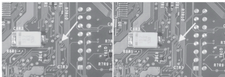
Figure E-1: Left, arrow points to the original pad that is being soldered. Right, pad has been torn off through excess heat and force.
